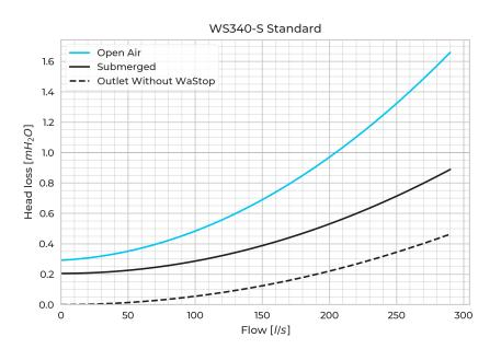
In the submerged case opening pressure [mmH2O /inH2O] is the difference between the water level upstream and the water level downstream and in the open-air case to the invert of the pipe. In vertical applications, the vertical opening pressure is measured from the outlet of the WaStop.
