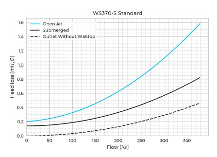
In the submerged case opening pressure [mmH2O /inH2O] is the difference between the water level upstream and the water level downstream and in the open-air case to the invert of the pipe. In vertical applications, the vertical opening pressure is measured from the outlet of the WaStop.
